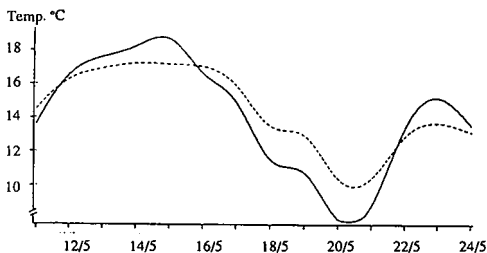
Fig. 4. Døgnet's middeltemperatur i 5 cm's dybde i kar og mark. 1988. — kar, - - - - mark. Mean of 24 hours soil temperature at 5 cm depth in containers and in the field. 1988. — containers, - - - - field.
