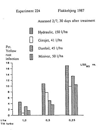
The result is to be considered as an example only. Rigid crops may give another result. Minivariant offers many possibilities of adjusting the direction of the nozzles and the air velocity. Danfoil and Minivariant operate according to very different principles. Tests conducted in 1986 showed that drifting was greater with Danfoil than that with an ordinary field sprayer. A test conducted in 1987 shows a very significantly reduced drifting with Minivariant, Fig. 4. The testing is being continued.
