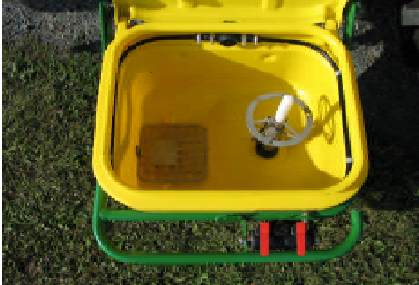
Fig. 8: induction bowl with circular rinsing pipe and container cleaning device.
