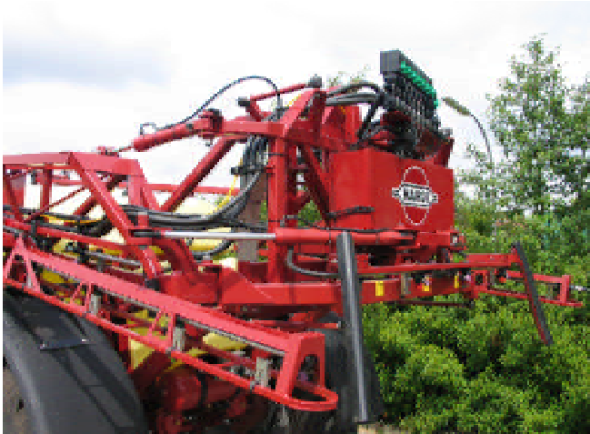
Fig. 6: boom suspension with section valve control unit
