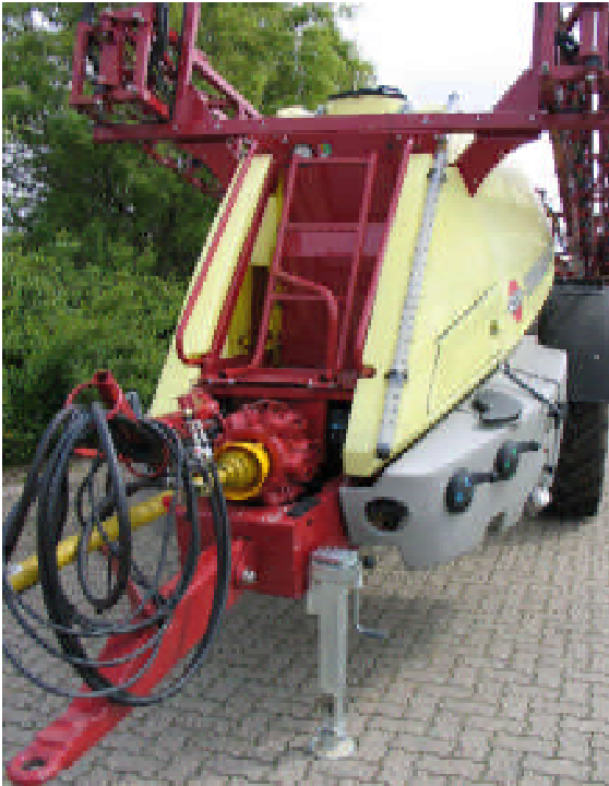
Fig. 4: rigid drawbar with trailer coupling ring for hitching, tank scale and operating controls.
