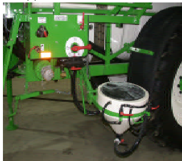
Fig.7: induction bowl in working position.
