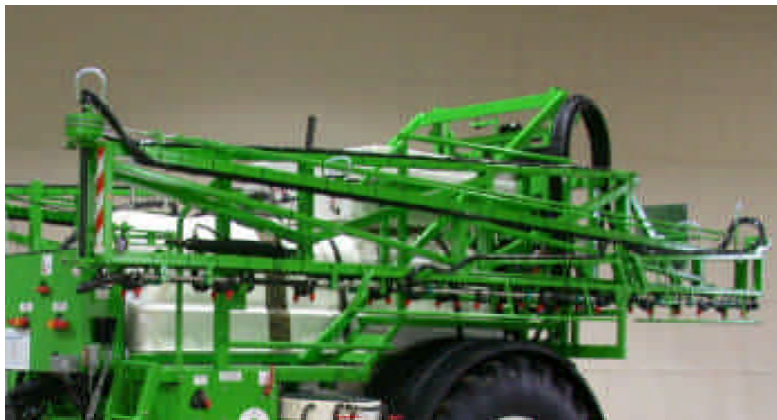
Fig.4: spray boom with stainless steel nozzle pipe.
