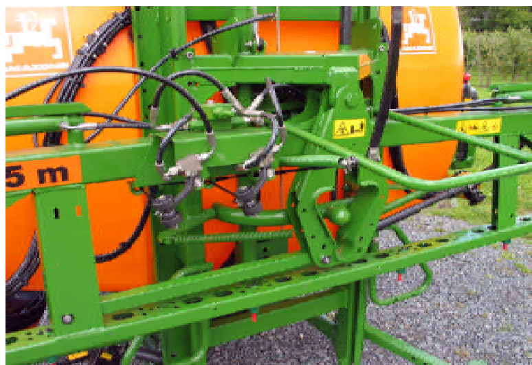
Fig.7+8: 15 m Q-plus boom which folds at the back, hydraulic on-off valves, hydraulic pendulum locking and spring-damping system.
