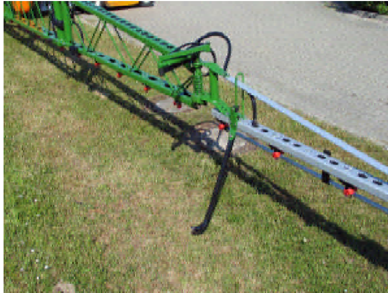
Fig.13: outer boom segment made of aluminium with protection bar on the 24 m Super-S boom.
