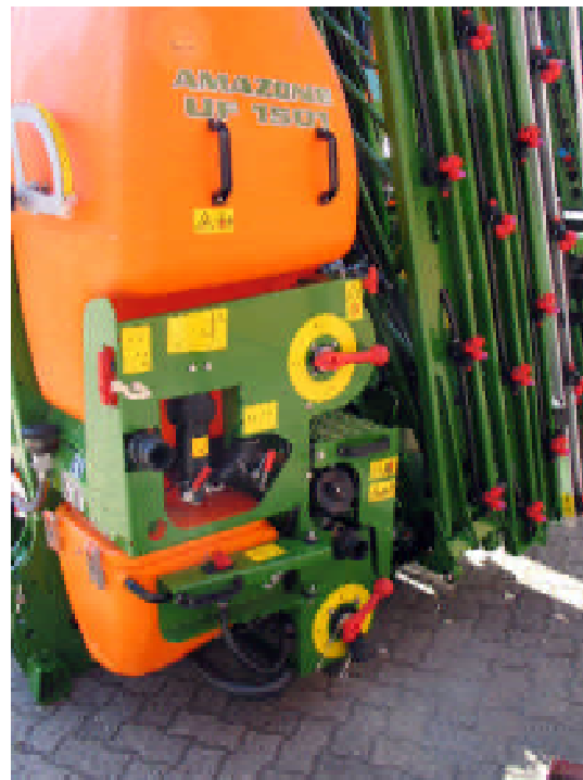
Fig. 4 operator panel with 5-way ball valve and filling connection on the left of the sprayer.
