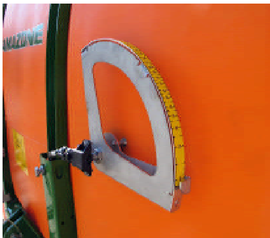
Fig. 2+3 castors and clean water tank (underneath the spray tank). Level indicator on the left at the front.
