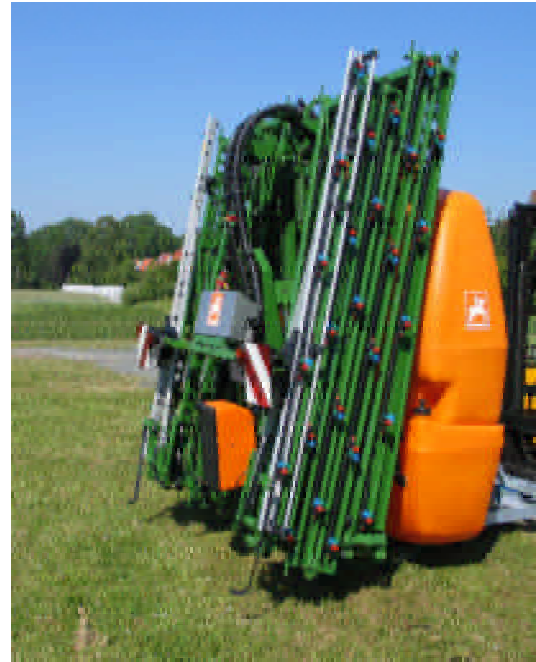
Fig. 10 : folded 28 m Super-S boom with section valve unit underneath stainless steel cover and tool box.
