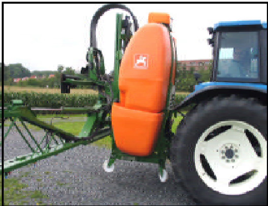
Fig. 2+3 castors and clean water tank (underneath the spray tank). Level indicator on the left at the front.
