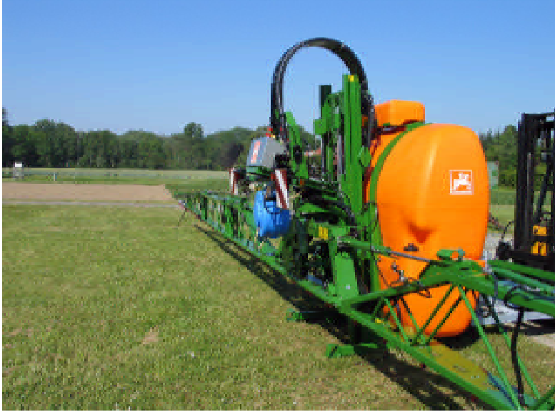
Fig. 12: non-buckling hose system leading to the boom.
