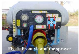
system, which uses water from an independent rinsing tank, can be controlled from the valves placed in front of the sprayer (figure 1). The hydraulic agitation system can be also turned on and
