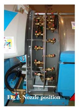
The sprayer is fitted with solenoid valves to turn on and off the boom sections (figure 2). There is a pressure compensating system for the two sides of the nozzle boom to prevent the working pressure from increasing, when the nozzles of one side are turned off. The electrical switchboard is also equipped with a manometer.
