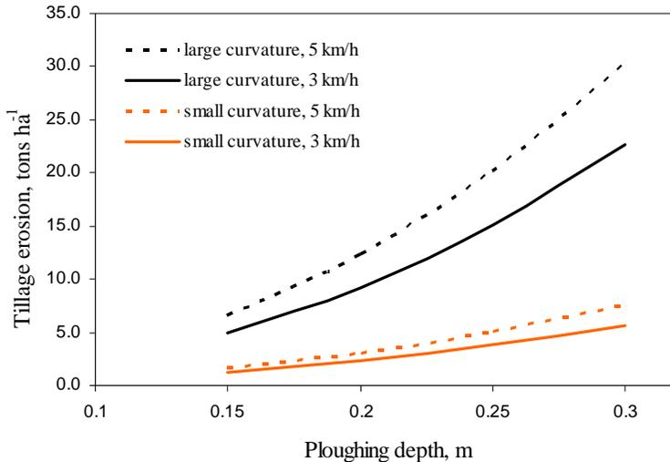
Figure 8.2. Predicted tillage erosion rates for mouldboard ploughing as a function of tillage depth, speed and topography. The tillage direction is parallel to the aspect and the soil bulk density  $1400 \text{ kg m}^{-3}$ . Based on Van Oost et al. (2006).
