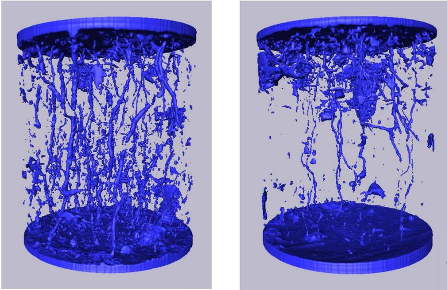
Figure 5.7. Macropores  $> \sim 0.5$  mm in undisturbed soil cores (20 cm height, 20 cm width) collected at 20–40 cm depth of a loamy soil in Skåne, Sweden, either with standard management (left) or trafficked four times by a heavy sugar beet harvester fourteen years prior to sampling (right). Preliminary results from the running inter-Nordic research project POSEIDON (<http://www.poseidon-nordic.dk/>). Digitized pictures created from Computer Aided Tomography (CT-scans) by Dorthe Wildenschild.
