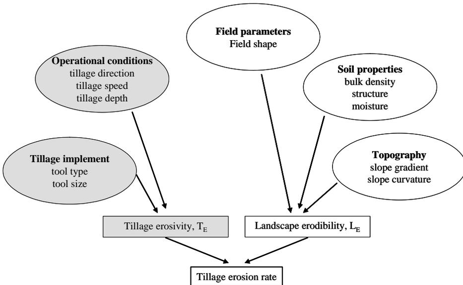
Figure 8.1. Factors affecting tillage erosion. The process of tillage erosion can be seen as a function of the erosivity of a given tillage operation ( $T_E$ ) and the erodibility of the cultivated landscape ( $L_E$ ). This simple general concept is the basis for the following discussion. Adapted from Lobb et al. (1999).
