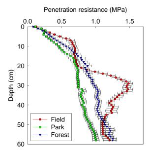
Figure 5.1. Cone penetration resistance measured at Barritskov Manor (loamy soil) in a non-trafficked park, a forest and in an agricultural field. Bars denote standard deviation (n=40) (Schjønning et al., 2000b).
