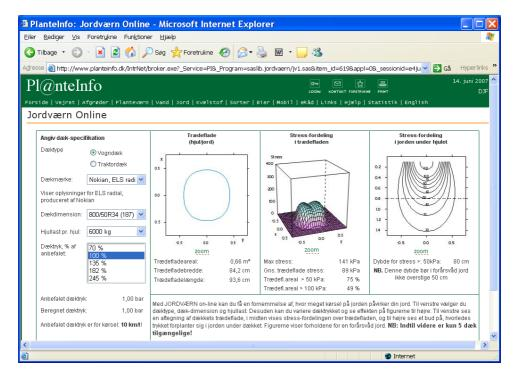
Figure 5.14. Features of the 'JORDVÆRN online' decision support system (prototype) showing diagrams of the contact area, the stress distribution in the contact area, and Söhne predictions of stresses in the soil beneath a selected tyre (www.planteinfo.dk, sheet 'Jord').
