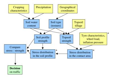
Figure 5.15. Route diagram illustrating the information flow in the planned decision support system 'JORDVÆRN online" allowing an evaluation of the sustainability of an intended traffic event on a specific field in Denmark. Please consult text for explanation of details. The boxes marked with an asterisk constitute the existing web tool (www.planteinfo.dk, sheet 'Jord').
