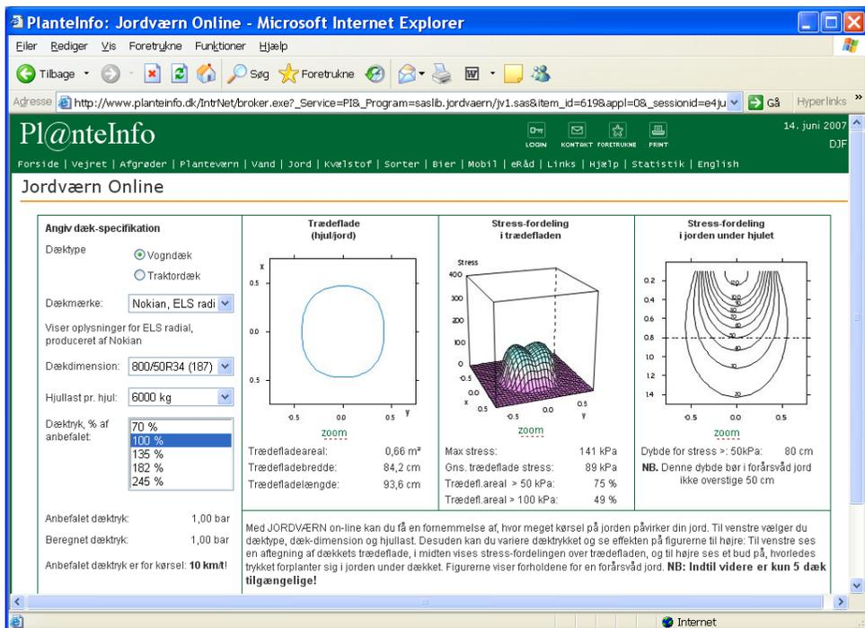
Figure 5.14. Features of the ‘JORDVÆRN online’ decision support system (prototype) showing diagrams of the contact area, the stress distribution in the contact area, and Söhne predictions of stresses in the soil beneath a selected tyre ([www.planteinfo.dk](http://www.planteinfo.dk), sheet ‘Jord’).
