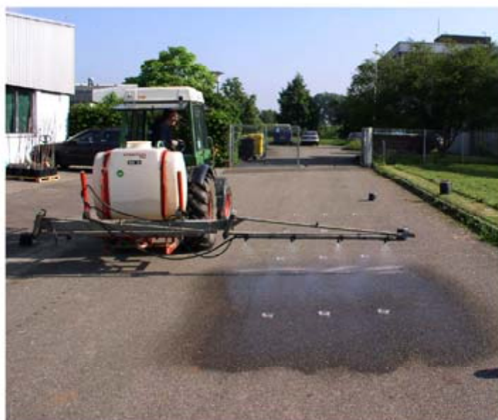
Figure 1. Spray equipment using a tractor-mounted spray boom for soil application of the nematode Steinernema feltiae against the cherry fruit fly in cherry plantations.
