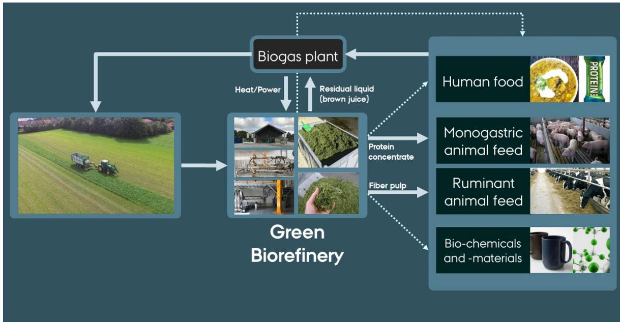
**Figure 2.1.** Sketch of the concept of green biorefinery, where grass is separated into a protein concentrate, a fibre pulp and a residual liquid (brown juice). Fully drawn lines denote already developed processes and the dotted lines processes under development (source: Morten Ambye Jensen).
