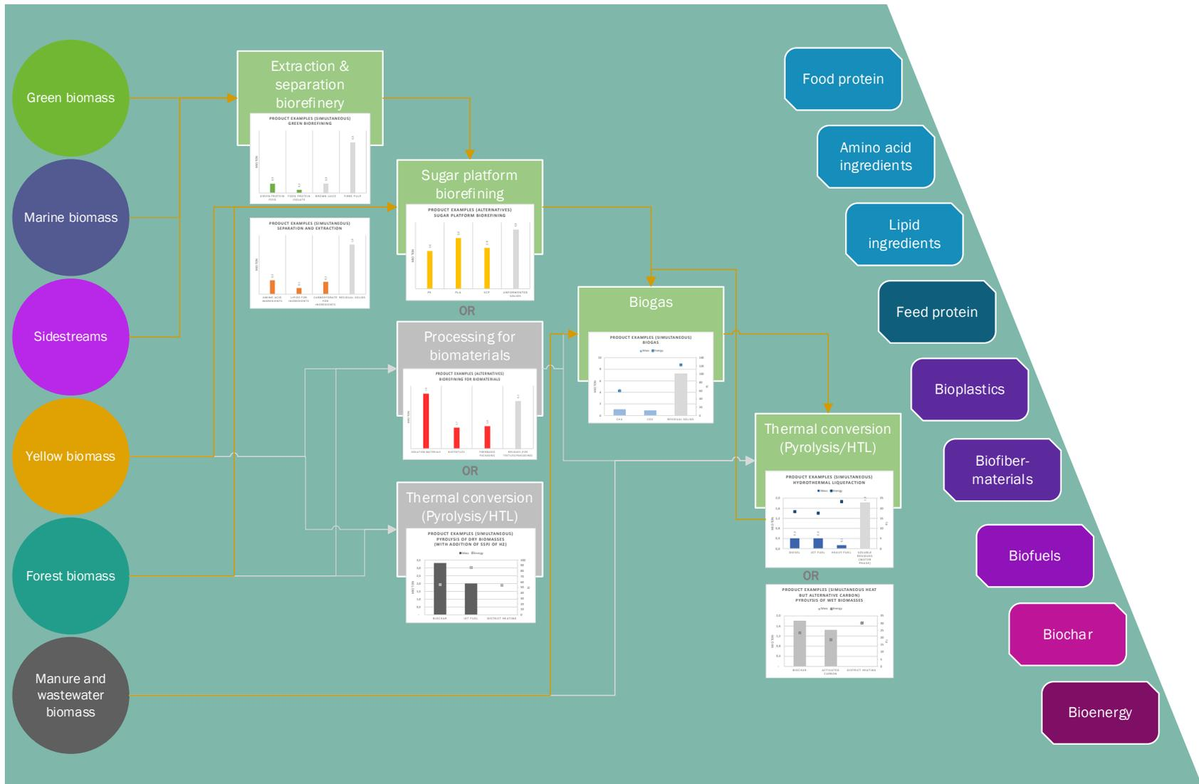
**Figure 5.11.** Biorefining system that cascades the bioresources. Yellow arrows draw a system for simultaneous process flows for inputs and outputs from different biorefining technologies. The grey arrows draw alternative process streams to alternative technologies for each bioresource and residual stream. On the left are the product categories that are possible to produce from such a biorefining system.
