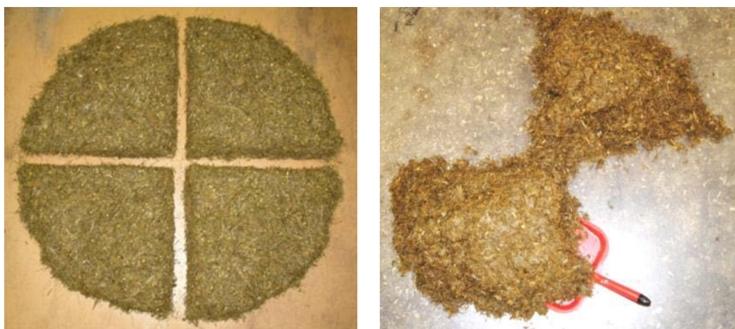
Figure 6. Feed sampling. Left: Feed sample mixed and divided in four quadrants. Right: remaining diagonal feed quadrants ready for further sampling (photo: Anon., 2014).
