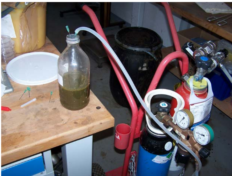
Figure 3. Flushing a batch test bottle with nitrogen to remove air in the headspace.
