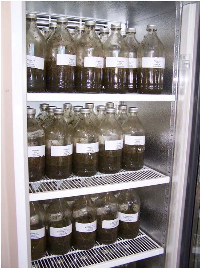
Figure 4. Batch assay bottles undergoing incubation.
