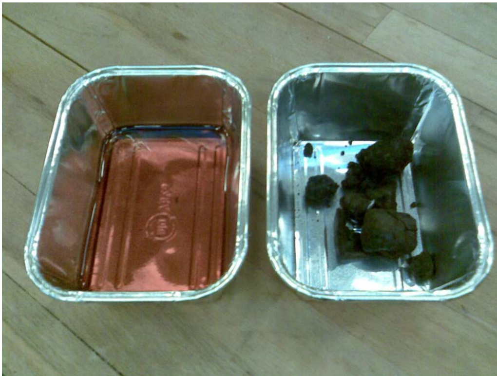
Figure 2. Samples of soapstock (left) and bleaching earth (right) showing the fluid nature of soapstock at room temperature (about 20°C), and the clay-like appearance of bleaching earth.
