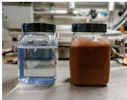
Figure 4.7. Picture of the two outputs from nanofiltration of residual juice. Left is the permeate going through the membrane. Right is the retentate, which is retained by the membrane. (Source G. Tirunehe, manuscript in prep)
